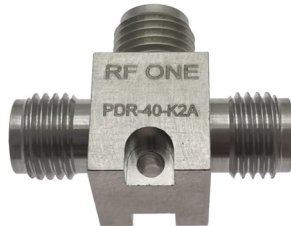
DC-40GHz, 2 Way 2.92mm Resistive Power Divider PN: PDR-40-K2A
